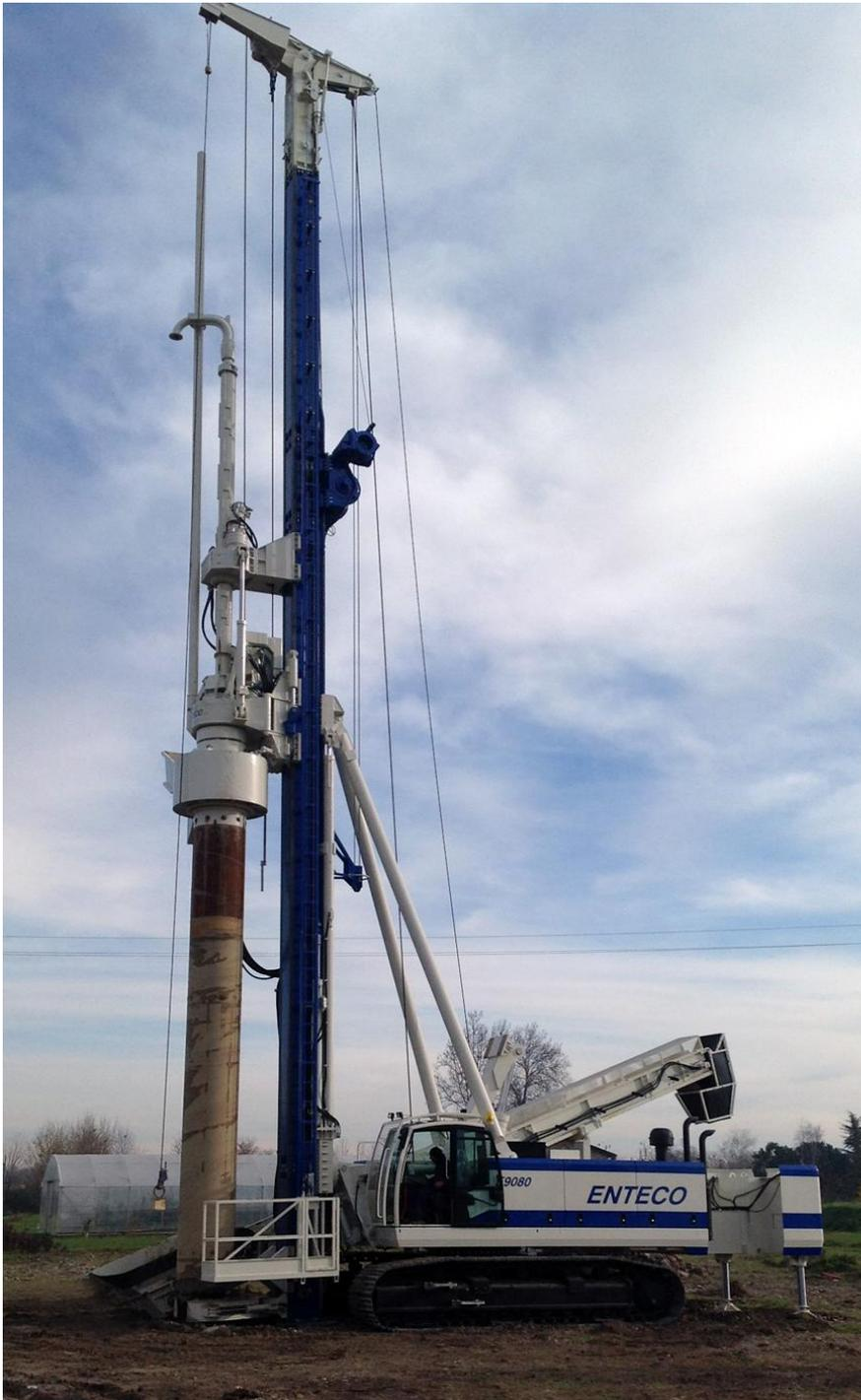
**ENTECO** high productivity hydraulic rig **E9080** is now available with a new double rotary assembly for **cased CFA drilling**, especially designed for secant piles with casing protection, **and a revolutionary patented system for recovery and discharge of the excavated material.**
